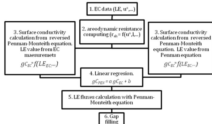
**Fig. 3.** The diagram of the procedure of filling the gaps in the database of latent heat flux values (LE)
