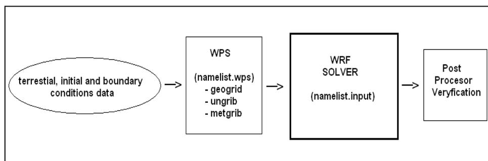
**Fig. 1.** Simplified idealized WRF system components
