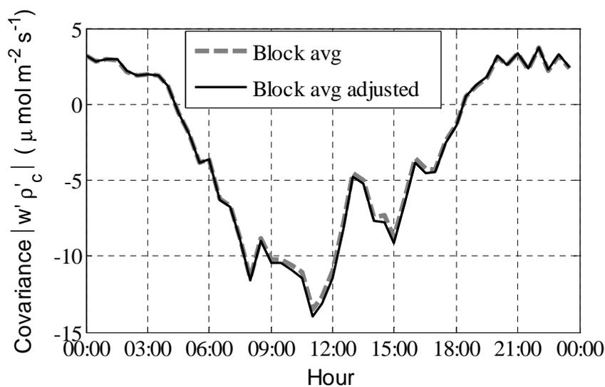
**Fig. 7.** Comparison of  $\overline{w'\rho'_c}$  covariances calculated on the basis of unprocessed measurement data (Block avg.) and after their moving in order to find the biggest quantity (Block avg. adjusted)
