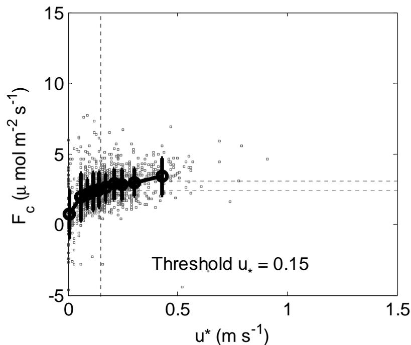
**Fig. 4.** The dependence of the quantity of  $F_c$  flux measured at night in Rzecin on the friction velocity ( $u^*$ ), for the months from June to August 2004. The upper dotted line shows the average  $F_c$  quantity calculated on the basis of the quantities measured above  $u^* = 0.15 \text{ m s}^{-1}$ . Lower line shows  $F_c$  quantity at the threshold quantity of  $u^*$
