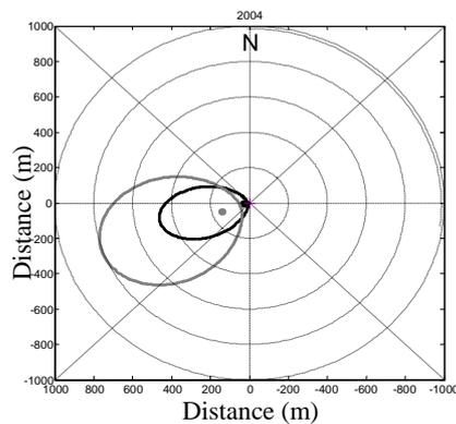
**Fig. 6.** Estimated footprint areas for 2004 by means of analytical method. Grey ellipse shows nighttime (windless periods), black one – daytime conditions with good turbulence). Grey point and a black point indicate the place of the highest influence on the measuring kit, for nights and days respectively. The sensor is located on the crossing of the lines in the middle of the map. Data gathered from April to September were used for the analysis
