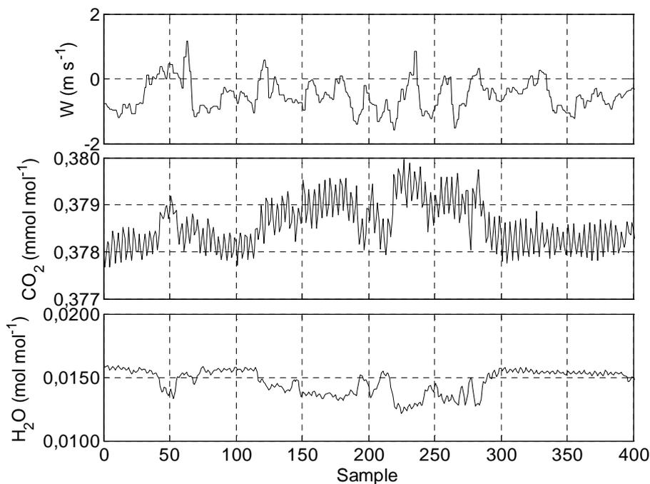
**Fig. 1.** Hypothetical course of the vertical component of wind velocity vector (upper graph), carbon dioxide concentration (middle graph), water vapor concentration (lower graph), in the ten-second measurement conducted at the frequency of 40 Hz. (On the basis of own measurements)
