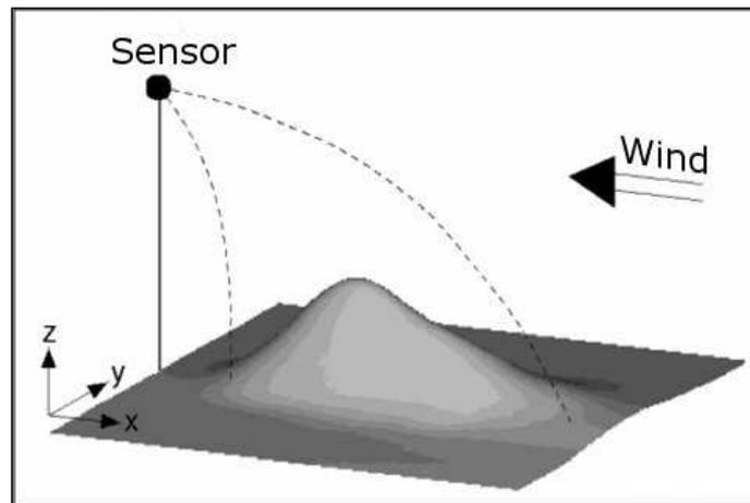
**Fig. 5.** Three-dimensional picture of the footprint obtained by means of Lagrangian stochastic model (dotted lines symbolize the boundaries of the atmosphere part which contains the trajectories of air which reaches the sensor) (Kljun *et al.* 2002)
