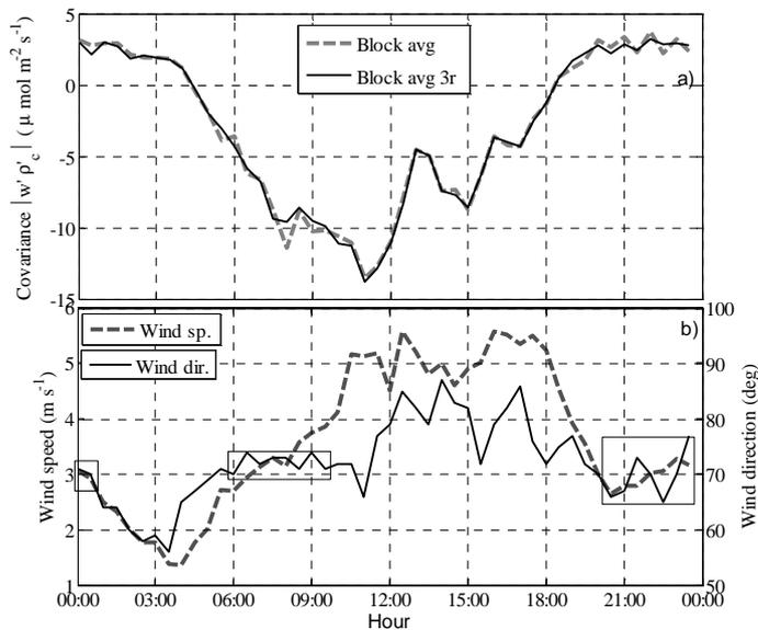
**Fig. 8.** Comparison of  $\overline{w'p'_c}$  covariances calculated on the basis of unprocessed measurement data (Block avg.) and after using the moving of measurement series and triple rotation (Block avg. Adjusted 3r)(a), the course of wind velocity and direction (b)
