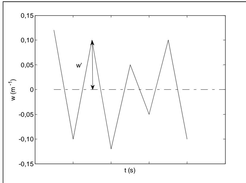
**Fig. 2.** Reynolds Decomposition for the vertical component of wind velocity ( $w$ ). red polygonal chain symbolizes measurement signal. Black dashed line shows a certain average in time ( $t$ ) from the measured values. Vertical arrowhead line shows aberration from the average ( $w'$ ).
