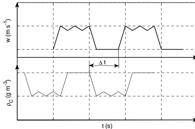
**Fig. 3.** A diagram illustrating the idea of moving measurement series against one another in order to obtain maximum covariance. Symbol  $\Delta t$  means the movement in time of data population „ $\rho_c$ ” against population „ $w$ ”, which is necessary to be introduced
