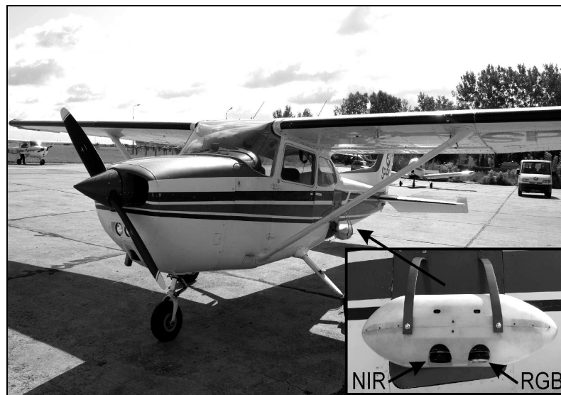
Fig. 2. Mounting the photo-platform on board the Cessna. NIR – infrared spectral channel, RGB – red, green, blue spectral channels (photo IUNG-PIB)
