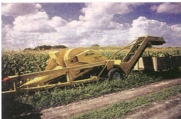
Rys. 5. Zbieracz kolb typu Pixall One-Row Pull Pix w czasie pracy [94] Fig. 5. Type Pixall One-Row Pull Pix cob picker during work [94]
