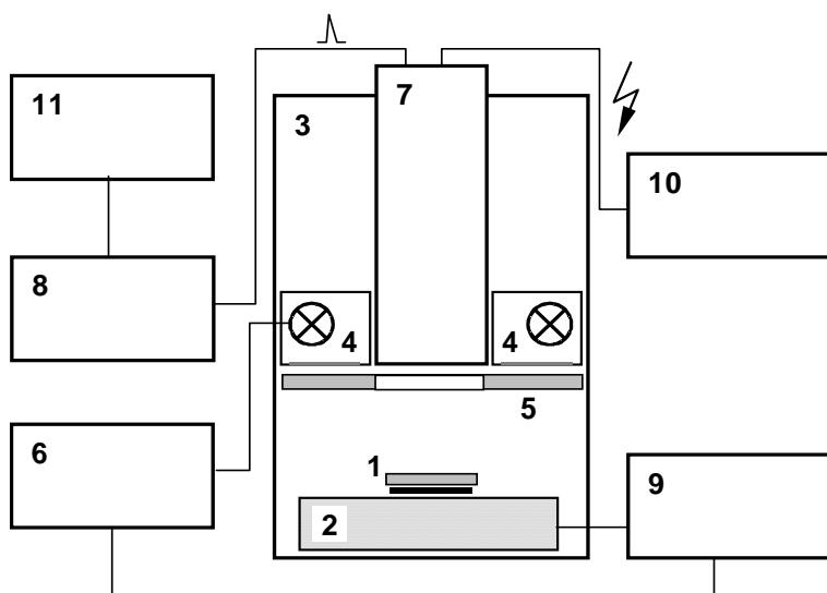
**Fig. 2.** Special luminometer for recording chlorophyll delayed luminescence decay
