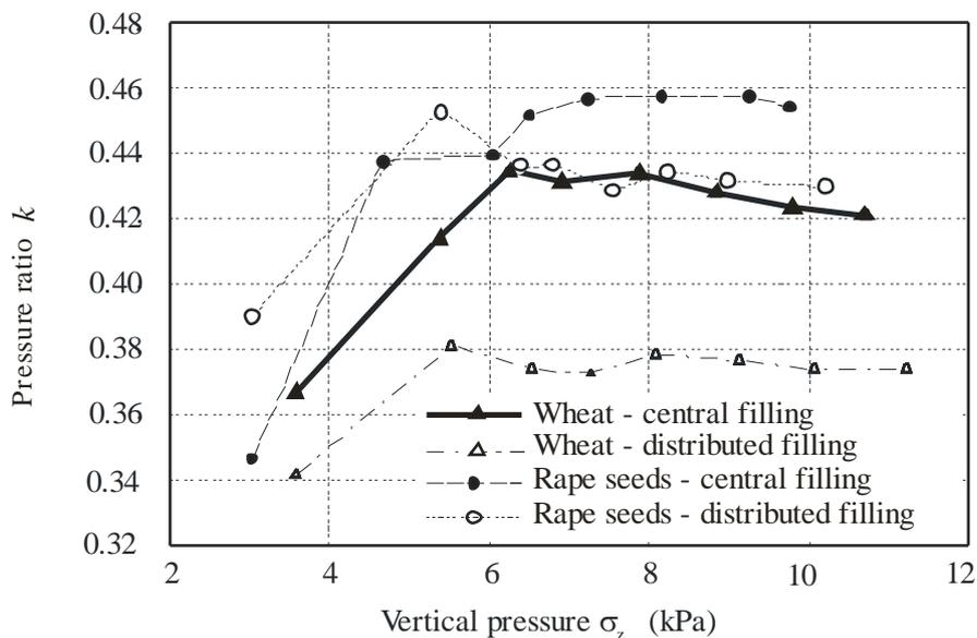
**Fig. 34.** Effect of the filling procedure on the pressure ratio determined on the model silo
