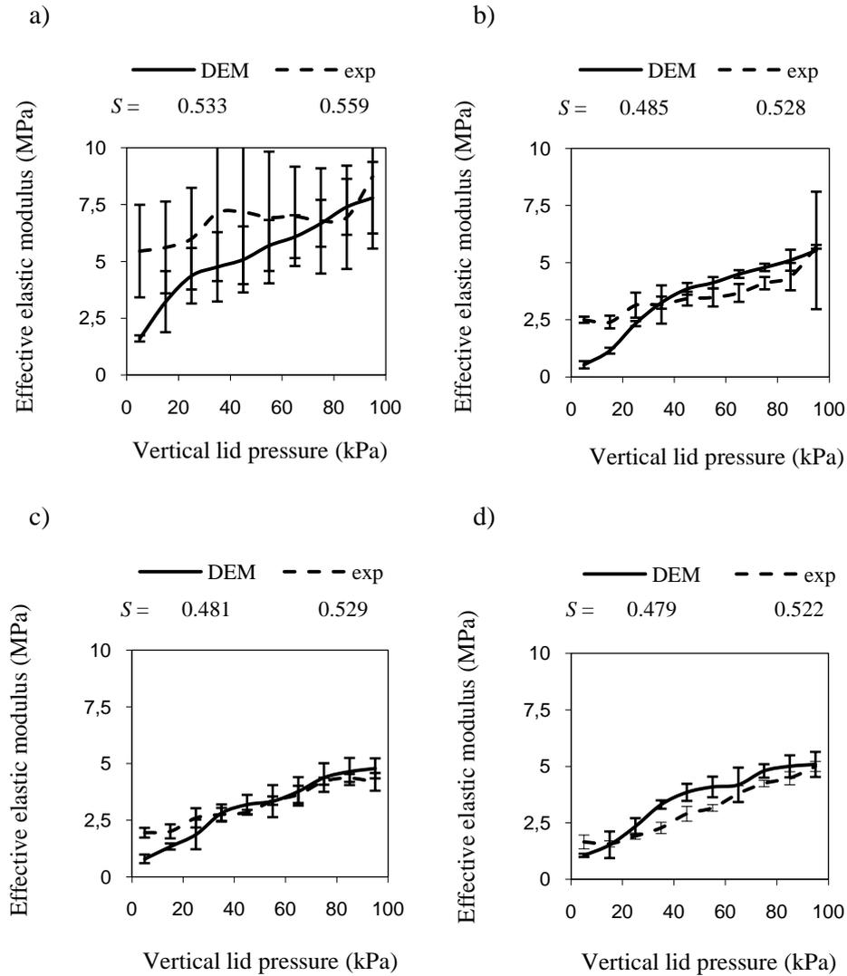
**Fig. 75.** Effective elastic modulus – vertical pressure relationships for numerical and physical samples of various thickness: a) –  $T = 8$  mm, b) –  $T = 21$  mm, c) –  $T = 33$  mm, d) –  $T = 44$  mm
