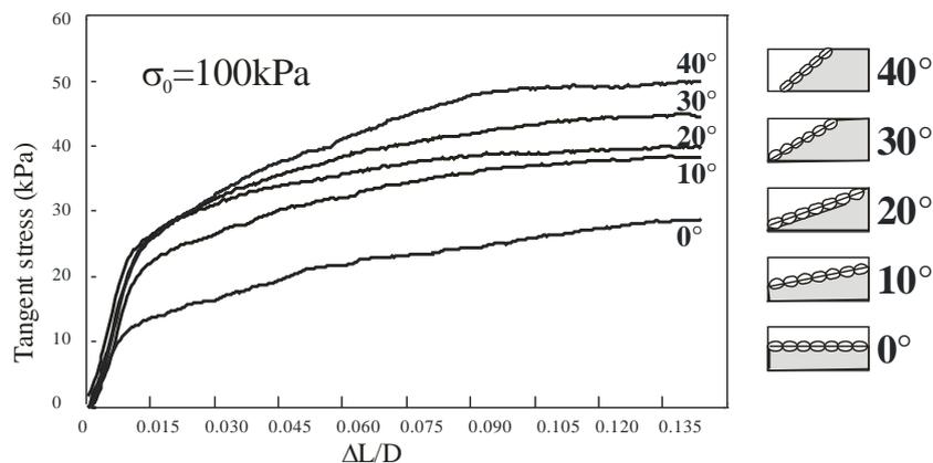
**Fig. 22.** Relationships of shear stress versus ratio of displacement to the sample diameter  $\Delta L/D$ . Samples of rye with an angle of preferred inclination of kernels long axes to horizontal ranging from 0 to 40 degrees (Molenda and Horabik 2005)
