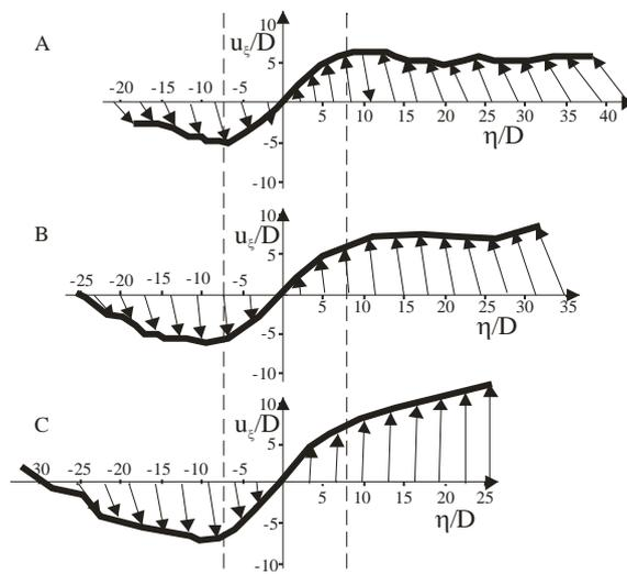
Fig. 25. Displacement distribution across shear band  $\varepsilon_l = 0.17$  (Horabik *et al.* 2000)
