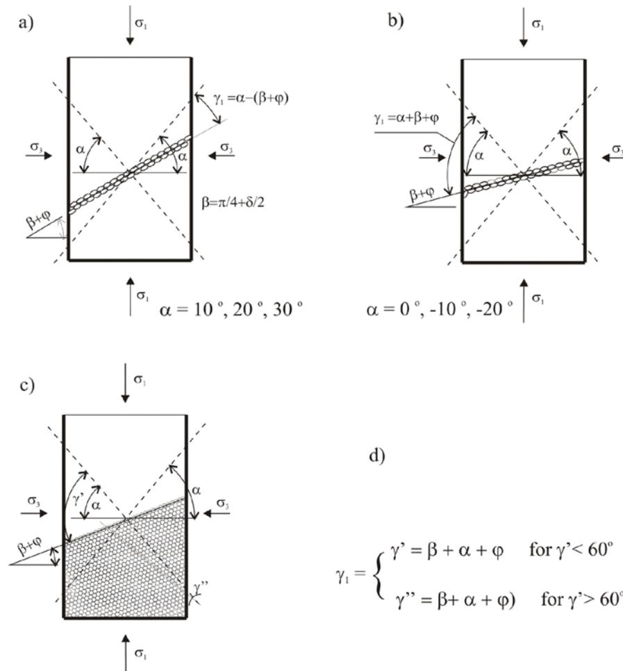
**Fig. 8.** Sample of granular material in triaxial compression test: a), b) – non-spherical grains, c) – spherical grains (Molenda and Horabik 2005)
