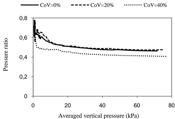
**Fig. 69.** The pressure ratio of specimen versus vertical pressure for sphere size variations of 0%, 20% and 40%
