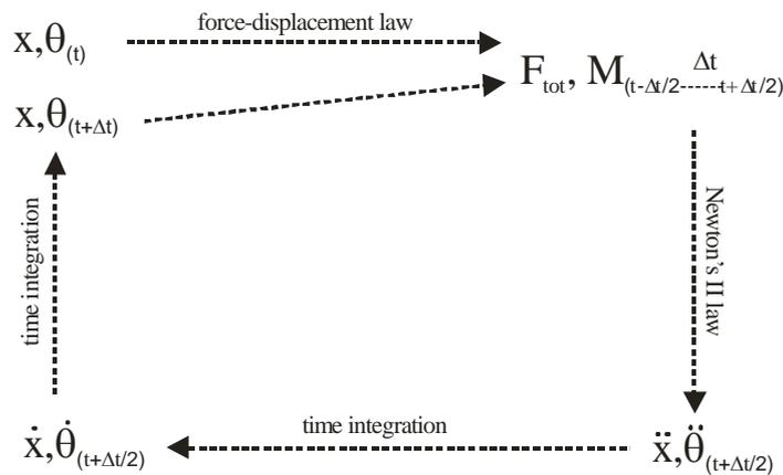
Fig. 51. Scheme of calculation cycle in DEM
