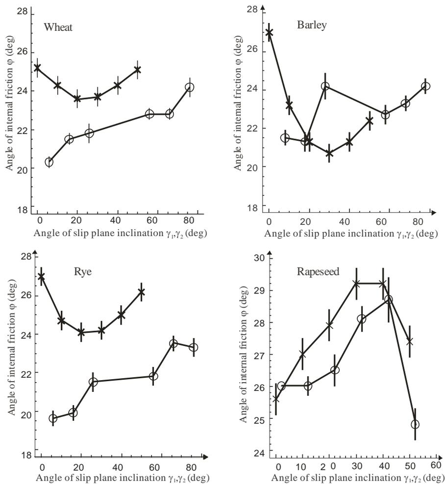
**Fig. 10.** Influence of the angle of slip plane inclination  $\gamma_1$  and  $\gamma_2$  on the angle of internal friction  $\varphi$  in direct shear test  $\times$  and triaxial compression test (Molenda and Horabik 2005)
