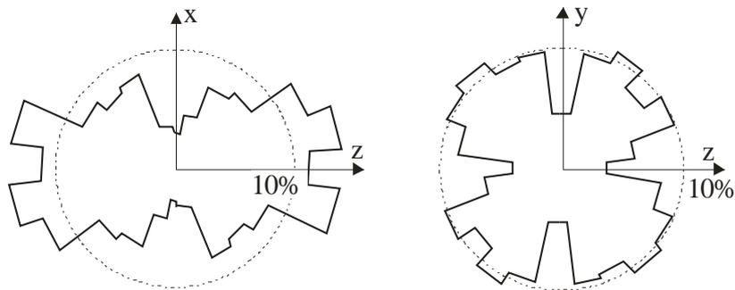
**Fig. 3.** Distribution of density of probability of angle of inclination to horizontal line of long axis of sand grains (Oda 1976)
