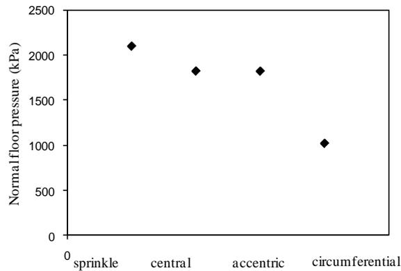
**Fig. 83.** Normal floor pressure for different filling methods
