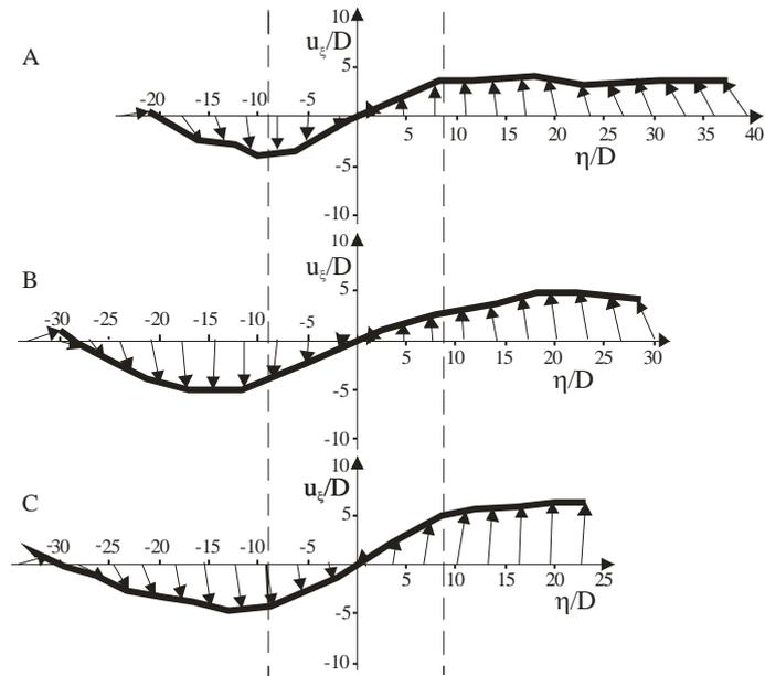
Fig. 24. Displacement distribution across shear band  $\varepsilon_l = 0.1$  (Horabik *et al.* 2000)
