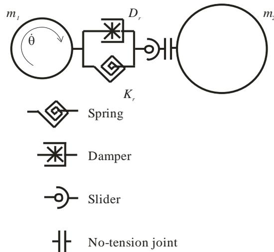
**Fig. 48.** Viscoelastic contact model with rolling friction (Iwashita and Oda 2000)
