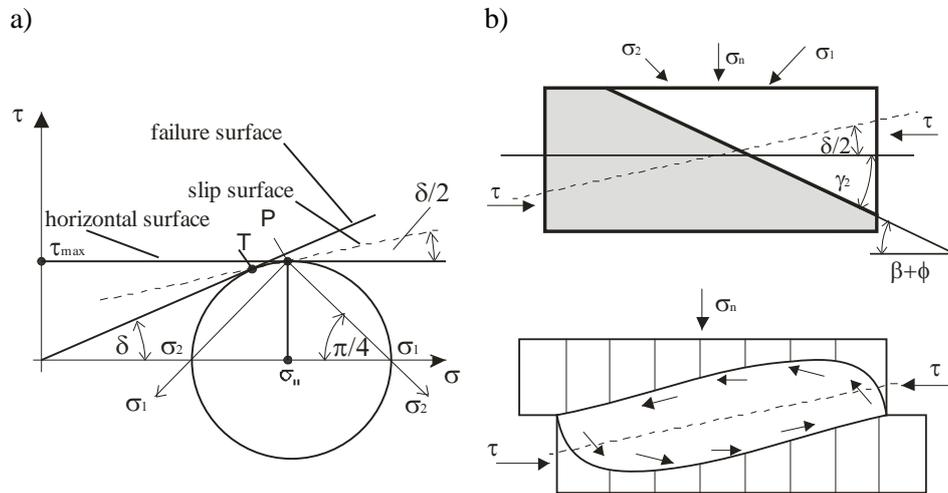
**Fig. 9.** Sample of granular material in direct shear test: a) diagram of Mohr for state of stress in the sample, b) orientation of preferred direction of long axis of grains against theoretical slip plane  $\gamma_2$ , c) image of deformation of the sample (Molenda and Horabik 2005)
