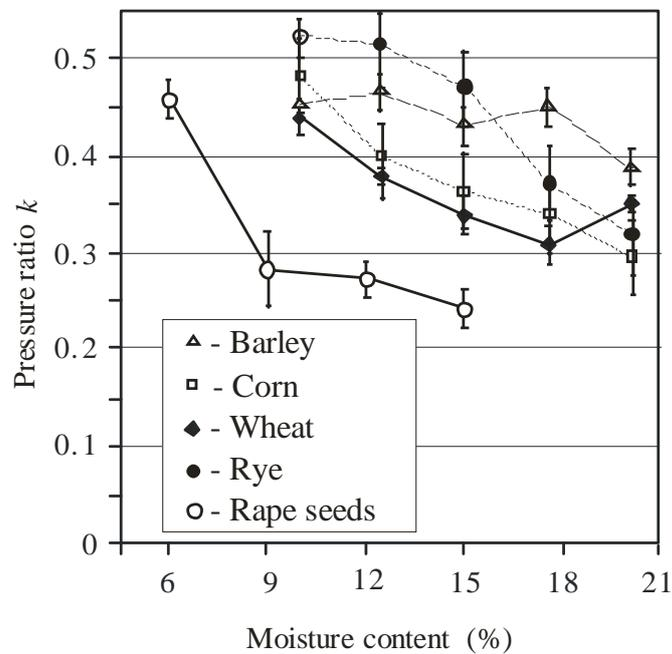
Fig. 35. Pressure ratio as influenced by moisture content of grain
