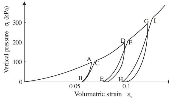
**Fig. 12.** Stress-strain relation during loading-unloading cycles of wheat grain in oedometric test (Molenda and Horabik 2005)
