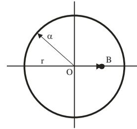
**Fig. 40.** Pressure applied to a circular region; displacement at a point B (Johnson 2004)
