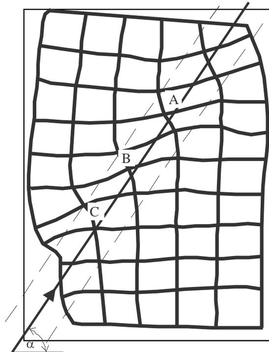
**Fig. 23.** Cross-section of mustard seeds sample deformed in triaxial compression test showing localization of deformation as shear band (Molenda and Horabik 2005)
