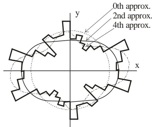
**Fig. 5.** Probability density distribution of angle of inclination of contact normals and their approximations (Kanatni 1984)
