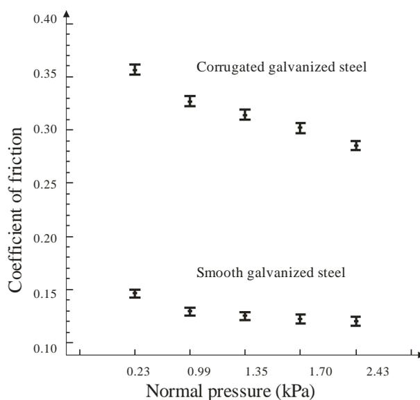
**Fig. 29.** Coefficient of friction of wheat on smooth and corrugated galvanized steel determined using tilting table method. Mean values and 95% confidence intervals for five levels of normal pressure (Molenda *et al.* 2000) normal pressure
