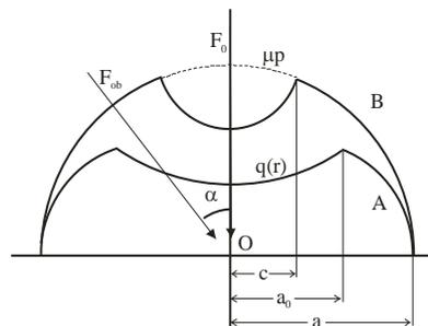
**Fig. 47.** Circular contact subjected to a steady normal load  $F_0$  and an oblique force  $F_{ob}$ . A – no micro-slip; B – slip in annulus  $c$  (Johnson 2004)
