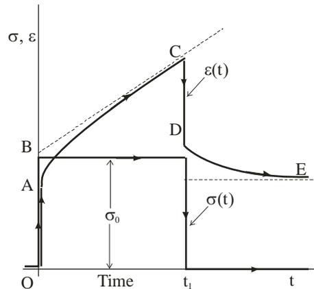
**Fig. 46.** Relationship between the strain in a specimen of viscoelastic material under the action of constant stress (Johnson 2004)
