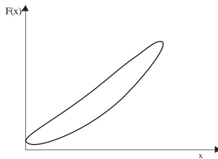
**Fig. 45.** Force-displacement relationship for viscoelastic contact between spheres
