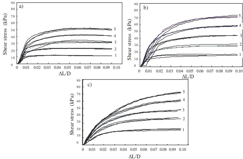
**Fig. 19.** Shear stress  $\tau$  versus ratio of displacement to the sample diameter  $\Delta L/D$  for wheat of moisture contents of: a) 12%, b) 20% and c) 22%, for normal stress  $\sigma_n$  of: 1-20 kPa, 2-40 kPa, 3-60 kPa, 4-80 kPa and 5-100 kPa (Molenda and Horabik 2005)
