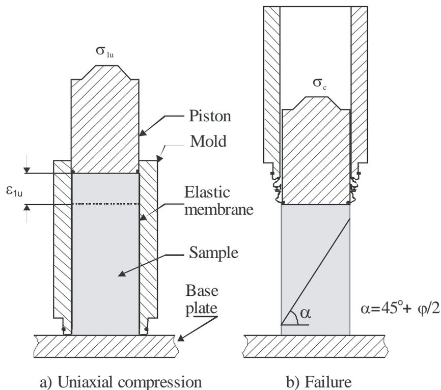
Fig. 39. POSTEC uniaxial tester (Maltby and Enstad 1993)
