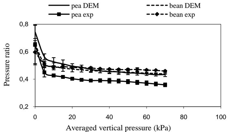
**Fig. 66.** Pressure ratio-vertical pressure curves for spherical and non-spherical seeds obtained from numerical and physical experiments
