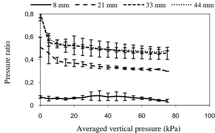
Fig. 74. Lateral-to-vertical pressure ratio in numerical samples of various thickness
