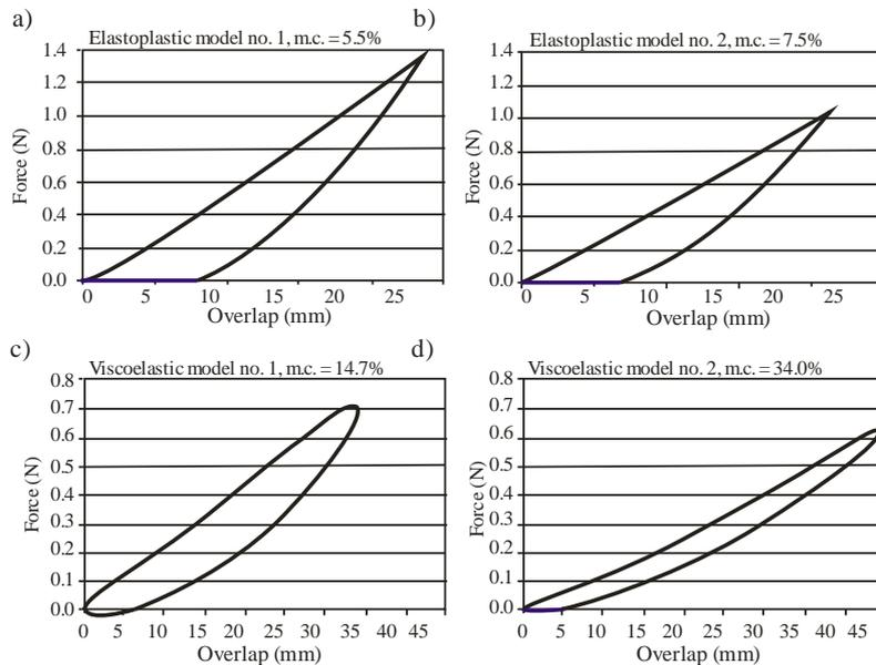
**Fig. 61.** Force-displacement relationship obtained from DEM simulations for elastoplastic and viscoelastic models
