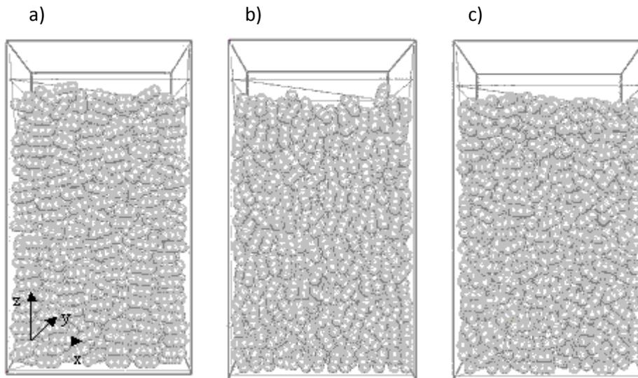
**Fig. 70.** Initial configurations of specimens composed of horizontally a), vertically b) and randomly oriented particles c)
