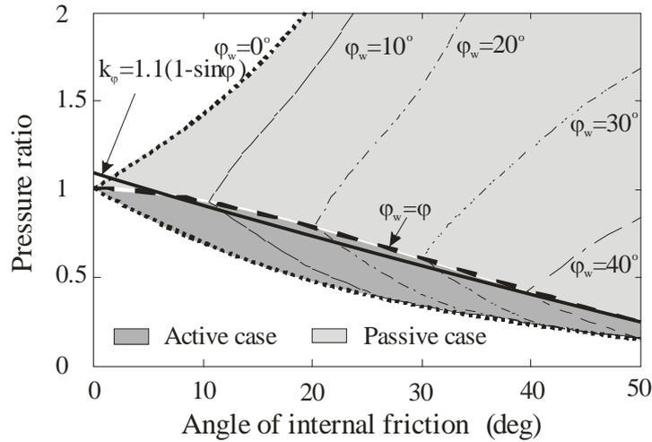
**Fig. 31.** Pressure ratio as a function of the angle of internal friction and the angle of wall friction for yielding at the wall in the active and passive cases (Horabik *et al.* 2000) — the pressure ratio according to Eurocode 1 (2003)
