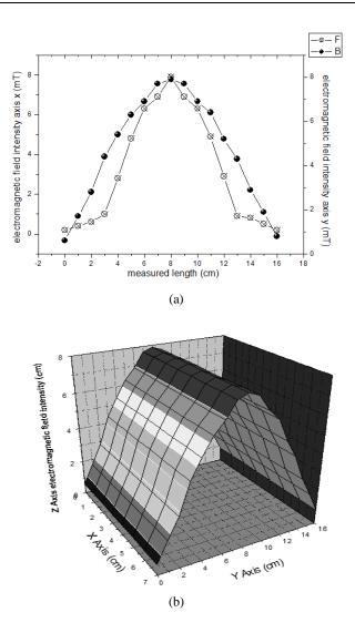
Fig. 3. Electromagnetic field distribution along axes "X" and "Y"
