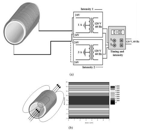
Fig. 2. Prototype irradiating of the electromagnetic field
