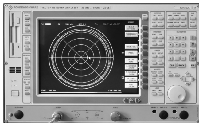
Fig. 24. Vector Network Analyser used for determine dielectric permittivity of investigated soils
